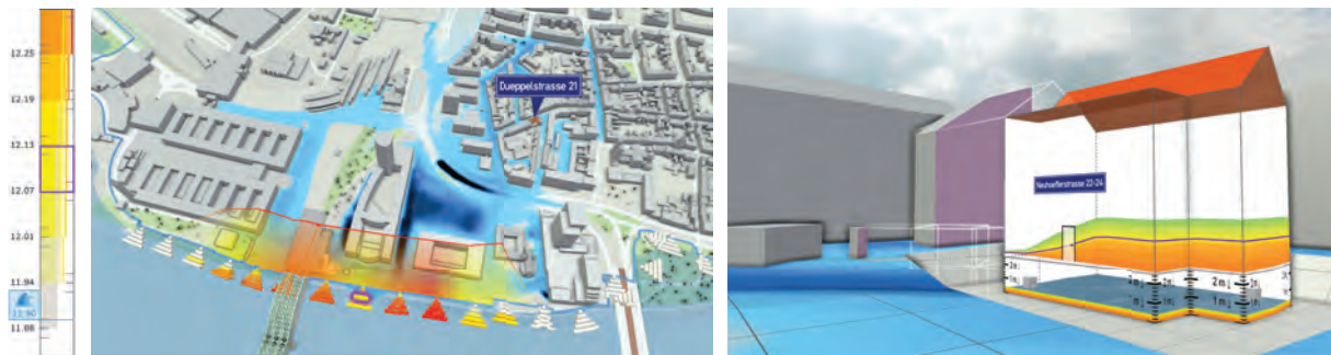
Figure 1: Understanding the uncertain vulnerability of a selected building to a multitude of flood scenarios. (Left) Vulnerability to floodwall overtopping events, displayed on a water gauge. (Middle) Vulnerability to floodwall breaches, shown along the protection wall. (Right) Adverse impact on the selected building, including cellar flooding. The probability of water reaching a particular level varies around the building and is mapped onto the facades.
