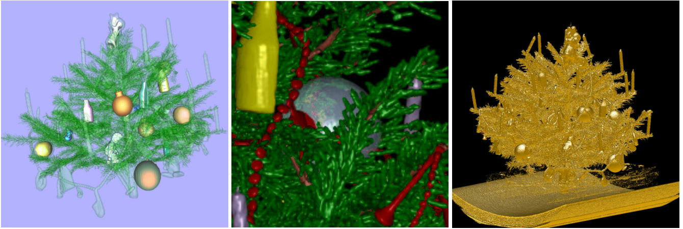
Figure 3: From left to right: OpenGL polygon rendering based on marching cubes surface extraction. Ray tracing of the segmented tree. Direct volume rendering: ray casting.
