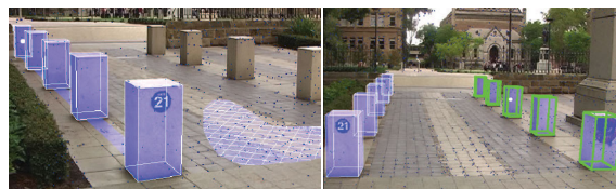
Figure 9: Interactive modeling of geometry in video. Left: Replicating the bollard by dragging the mouse. Right: Repeating a row of bollards. Figure courtesy of Anton van den Hengel [vdHDT*07a] ©2007 ACM.
