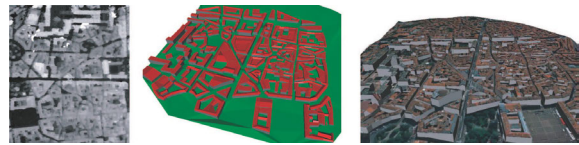
Figure 25: Automatic urban area reconstruction results from a DSMs (left): without (middle) and with textures (right). Figure courtesy of Florent Lafarge [LDZPD10], ©IEEE 2010.
