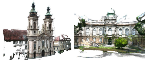
Figure 23: Examples of dense reconstruction after depth map fusion. Figure courtesy of Arnold Irschara [IZB07], ©2007 IEEE.
