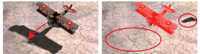
Figure 4: Shadows from moving object. Left: Correctly shadowed scene of a moving toy airplane using PCSS. Right: Naive reprojection using depth comparison only recognizes that the shadow on the airplane needs to be updated, but does not indicate the need for a shadow recalculation in the regions marked with red ellipses.
