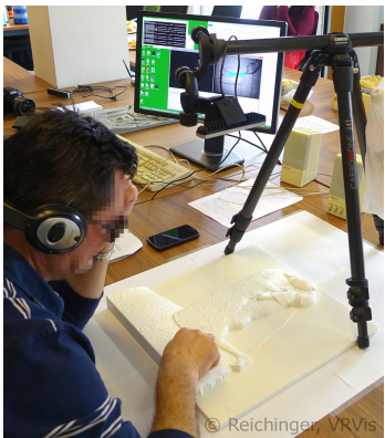
Figure 7. A participant explores the Gesture-Based Audio Guide during the Vienna evaluation. The depth camera tracks the users' gestures, which are interpreted by a custom software running in the background.
