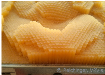
Figure 5. Close-up of the spaghetti pin matrix. Note the rough edges of the cylindrical ends.
