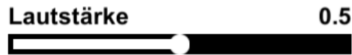
Figure 4.9: Example slider used in the GUI. Slider with round handle due to the round button GUI design. Starts in the middle. On top there are two texts explains what can be changed - Lautstärke (Volume) - and the adjusted value - 0.5 .
